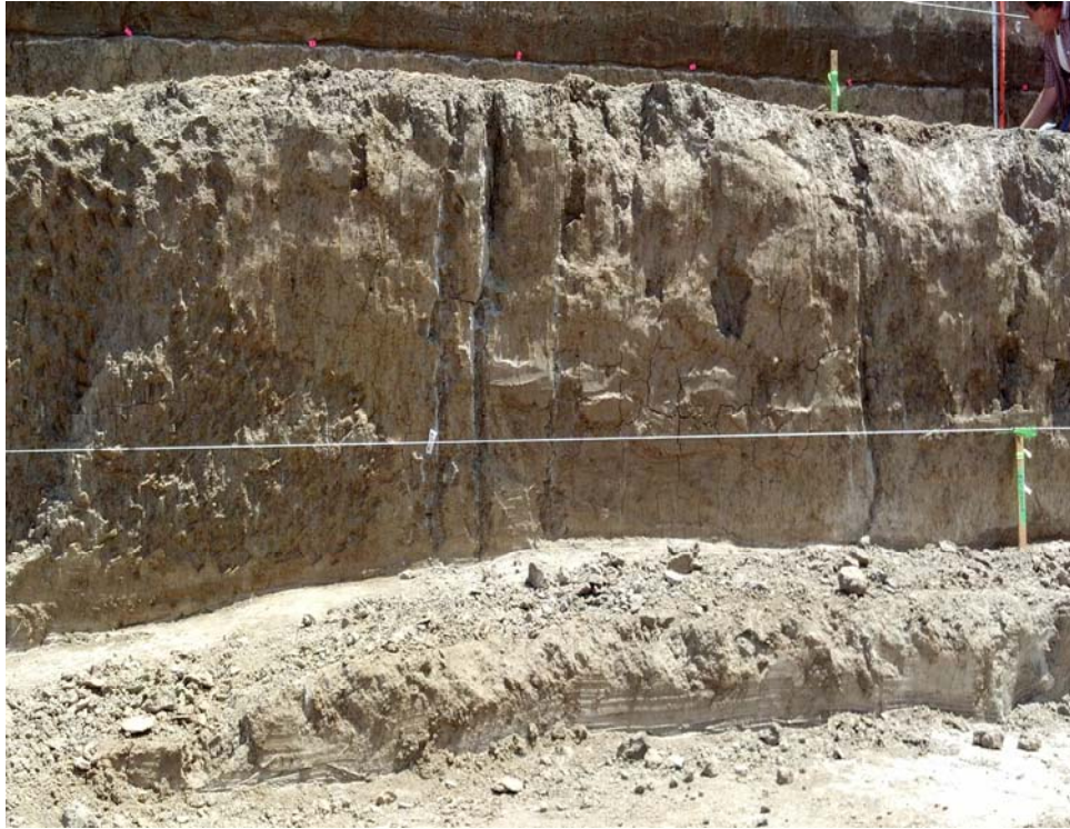
Photo 17 – Discontinuous Fractures – Station 0+50
